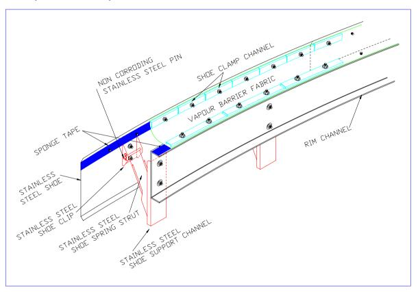
The **BTE** Shoe Seal vapour barrier fabric can be reinforced urethane, PVC/NBR, or glass reinforced PTFE. Essential metal parts are made in 304 grade stainless steel, with use of aluminium for some components, for lightness.
